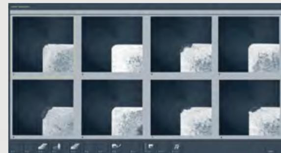
Fully automatic single image recording of the cutting edges at incident light for checking wear.
