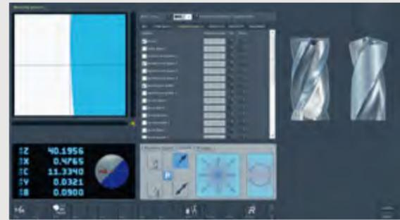
For measuring the chip space, the circumference (see above) and the face of tools. The measuring procedures and parameters can be freely defined and selected individually via the Checkbox.
