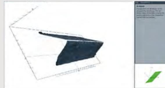
A 3D model of the scanned cutting edge is generated and outputted to evaluate the contour profile of the cutting edge preparation.
