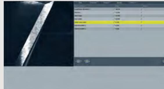
For the automatic determination of tool contours, radii, angles, distances, chamfer widths as well as wear and other parameters with incident and transmitted light.
