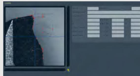
For fully automatic generation of measuring procedures and programs in »pilot 3.0«, including calculation of the intersection points, distances, angles and much much more.
