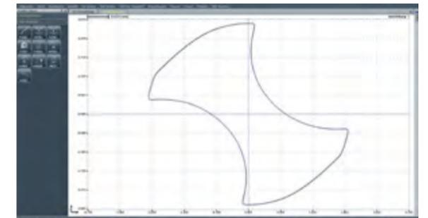
Micro-precise recording of contours via the ZOLLER »pilot 3.0« software function »lasso«, illustrated here for a drill section.
