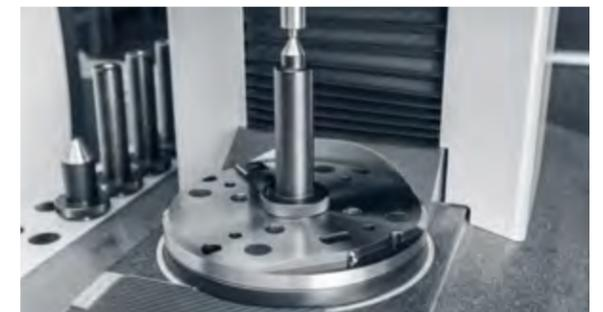
Precise positioning: the CNC-driven base spindle with rapid change interface for optional inserts and the pneumatic tailstock ensure precise clamping which is essential for accurate measurement.
