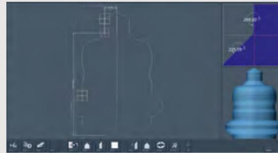
For the automatic generation of 2D sectional drawings or 3D (CAD) graphics from the measured actual dimensions on step tools or die plates.
