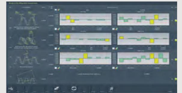
Detailed and graphic evaluation of cylindrical hob cutters according to DIN 3968. Documentation of the concentricity/run-out of the hub diameters, deviation in shape/position of the rake face, deviation in shape of the cutting edge/tooth thickness, flute direction and many more parameters, including grading of the quality class.
