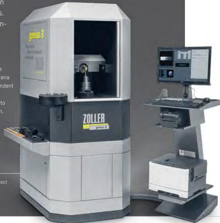
»genius 3s« with full housing to protect against dirt and extraneous light.
