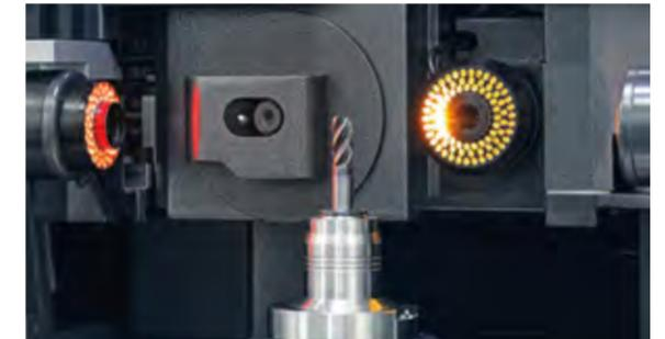
Measuring room »titan« with high precision spindle, with CNC swiveling device for optical carrier, CCD cameras and LED lighting.
