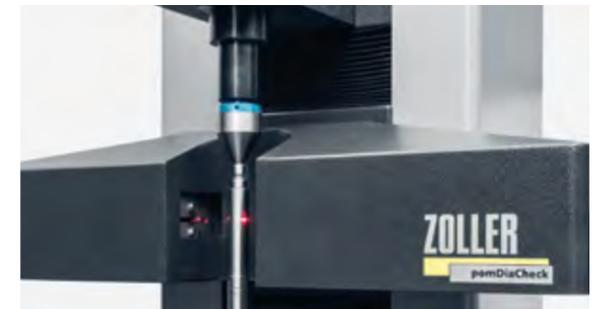
Laser micrometer for micro-precise measurement, contactless and close to production.
