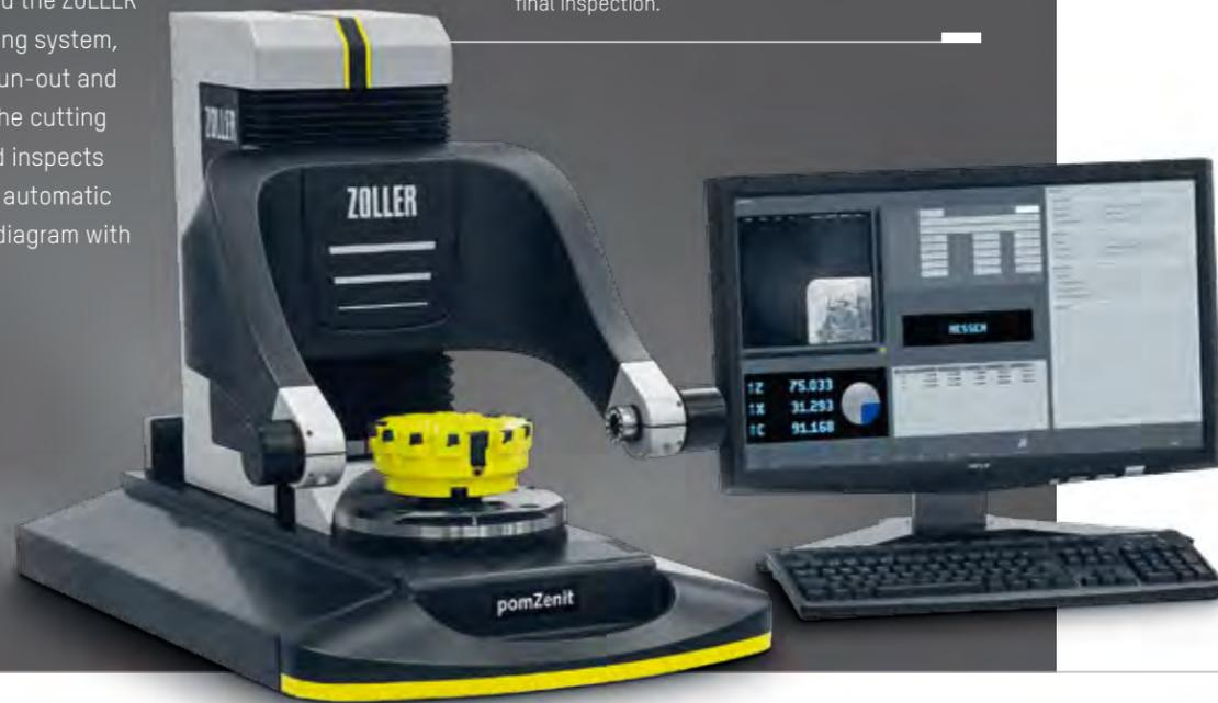
Measurement of all cutting edges including graphic display of measured results »focus 360°i«
