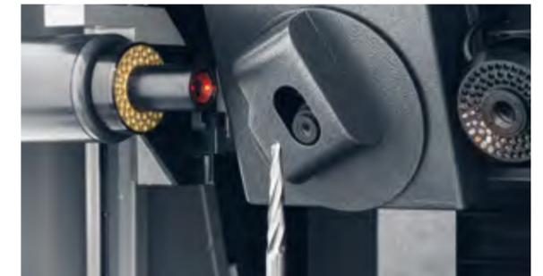
Measurement of edge rounding in the radius segment with CNC-swiveling »Z3dCam« sensor.
