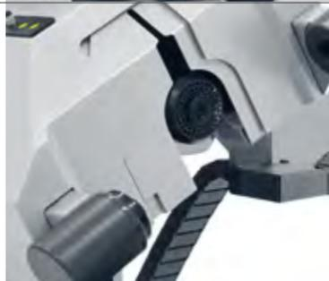
Micro sensor for measuring micro-geometries, i.e. protective and supporting chamfers.
