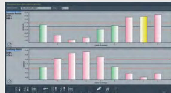
The software measures all cutting edges of a tool in a rotary manner and displays the measured values of every cutting edge graphically or in table form, including the tolerance range and fast remeasurement of individual cutting edges (yellow bar) directly from the diagram.
