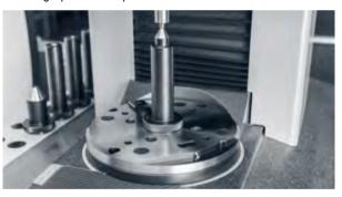
Precise positioning: the CNC-driven base spindle with rapid change interface for optional inserts and the pneumatic tailstock ensure precise clamping which is essential for accurate measurement.
