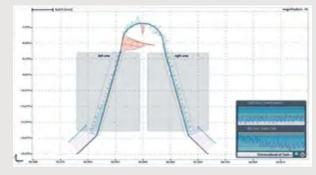
Evaluation of tooth form via variable measuring windows at the flanks, including automatic target-actual comparison.
