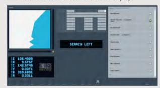
Automatic display of measuring status and scan taking pitch and rotation angle into account.
