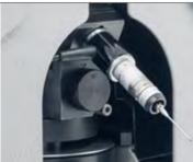
Swiveling optical carrier for distortion-free measurement and checking of helical tools with transmitted light.
