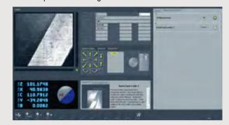
Live image and virtual joystick with navigator allow very easy definition of the measuring position.
