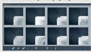
Fully automatic single image recording of the cutting edges at incident light for checking wear.
