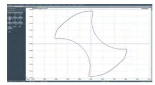
Micro-precise recording of contours via the ZOLLER »pilot 3.0« software function »lasso«, illustrated here for a drill section.
