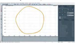
Determination of contour profile and transfer of target contour in »lasso« for thread formers.
