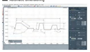
CAD function for generating and dimensioning the actual contours.
