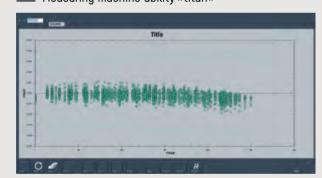
The certified FKM gauge, which can be traced to the national standard, automatically determines a range where the true value of the measured dimension lies, with a probability of 95%. A measuring uncertainty of at least E=1.8+ (L/250 mm) µm is achieved with the »titan«.
