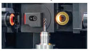
Measuring room »titan« with high precision spindle, with CNC swiveling device for optical carrier, CCD cameras and LED lighting.
