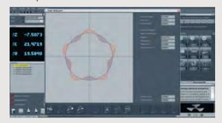
Graphical evaluation of the measurement results including tolerance range.
