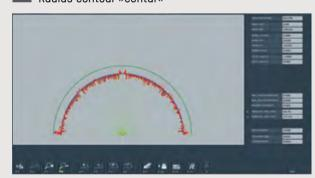
Fully automated determination of the cutting edge profile and radius and graphic evaluation of the entire contours with tolerance range and variable setting of the angle sectors.
