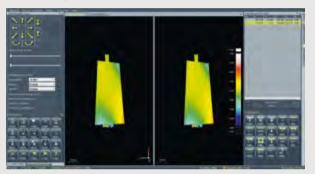
Fully automatic color coding of target-actual comparisons for any type of object, as illustrated for a turbine blade here.
