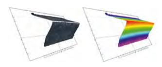
The cutting edge can be displayed in different modes – as texture for the immediate recognition of possible surface indentations and surface quality, or topographically to display the height profile of the cutting edge preparation at a glance.
