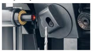
Measurement of edge rounding in the radius segment with CNC-swiveling »Z3dCam« sensor.
