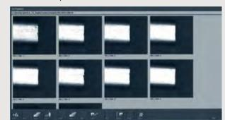
The »aec« function automatically records the circumferences of an optional number of teeth and thus provides a quick overview for finding and targeted checking of major wear to ensure that neither too little or too much is removed during resharpening.
