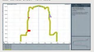
Scan, compare - finished! Whether drills, countersinks, milling cutters or cutting inserts: simply enter the start and end points, the scan is performed automatically and the actual contour is compared with the target contour with micro-precision.
