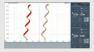
Measuring program for scanning tool contours and calculation of contour correction using the target DXF file of eroded or ground form tools. Output of the new contour is in DXF format.
