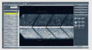
Live image of the cutting edge preparation for fast alignment and checking of surface.
