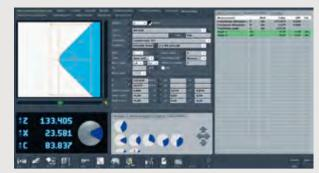
User interface »pilot 3.0« with automatic measurement of length, diameter, corner radius and cutting edge angle.
