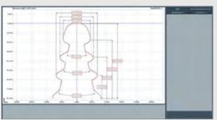
The actual contours are automatically dimensioned and evaluated in accordance with the given target contours.
