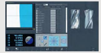
For measuring the chip space, the circumference (see above) and the face of tools. The measuring procedures and parameters can be freely defined and selected individually via the Checkbox.
