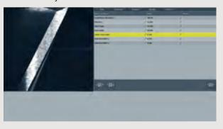
For the automatic determination of tool contours, radii, angles, distances, chamfer widths as well as wear and other parameters with incident and transmitted light.
