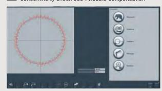
Fully automatic determination of concentricity with graphic analysis of the contour profile, including target-actual comparison and subsequent automatic concentricity and wobble compensation.
