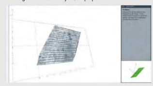
The contactless and automatically scanned tool surfaces can be displayed to give three-dimensional information on the calculation of the effective cutting angles or draft angles.
