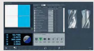
For measuring the chip space (see above), the circumference and the face of tools. The measuring procedures and parameters can be freely defined, selected via the Checkbox and saved for the tool.
