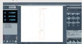
Highly accurate determination of diameters  $\lessdot 1$  absolute using the snap gauge principle.
