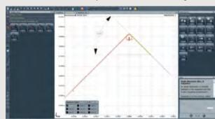
This function enables a target-actual comparison versus a DXF ideal contour including automatic dimensioning of the contour of the cutting edge.
