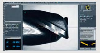
Determination of chamfer width and spiral angle.
