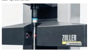
Laser micrometer for micro-precise measurement, contactless and close to production.
