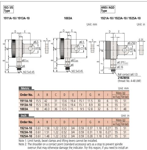
optional contact point with an outside diameter smaller than 7 mm, use a washer (with outside diameter of at least 7 mm, inside diameter of 3 mm, and thickness of approx. 0.5 mm) placed between the contact point and the spindle.
