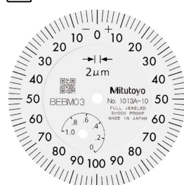
Graduation: 0.002 mm, Measuring range: 1 mm 1013A-10 Shockproof Jeweled bearing
