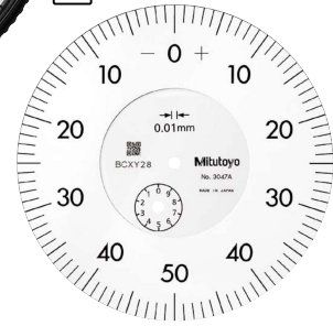
Graduation: 0.01 mm, 3047A Measuring range: 10 mm
